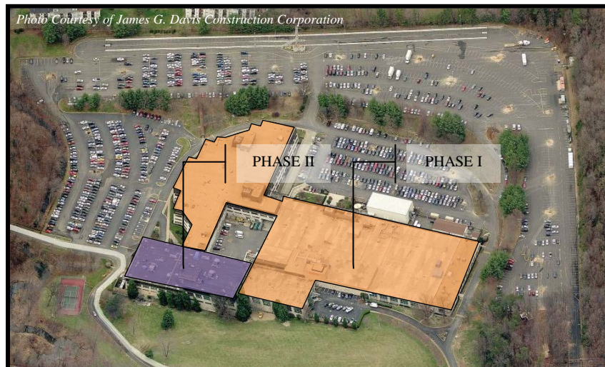
Figure 1 | 2-phase Construction Sequence
